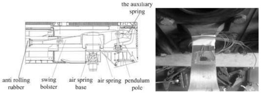
Fig.1The secondary system of the high speed maglev vehicleFig.2Arrangement of measuring points
